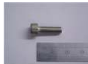
2. SP 001 009 SCREW, M5 x 16MM SOCKET CAP
